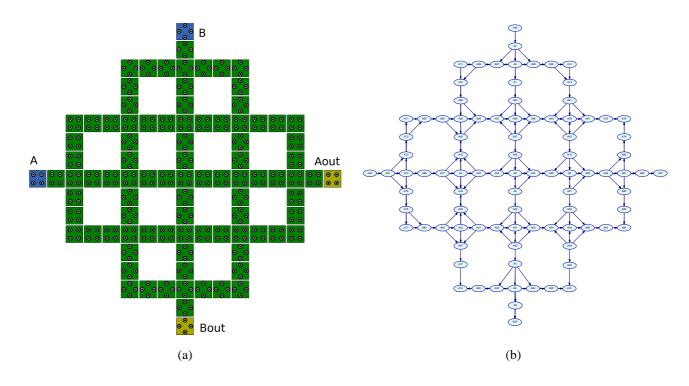
Fig. 8. 3 x 3 TMR crossing with rotated central cell (a) Layout (b) BN with 2-cell radius of influence.
