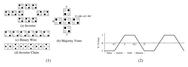
Fig. 2. (1) Basic QCA devices (2) Cmos-Clock-Signal
