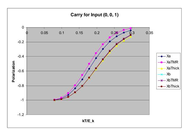
Fig. 19. Full Adder: Thermal performances on the carry output
