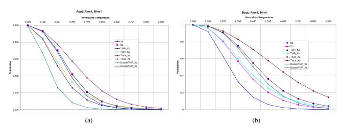
Fig. 15. Output polarization vs normalized temperature for A=1 B=1 (a) Aout (b) Bout
