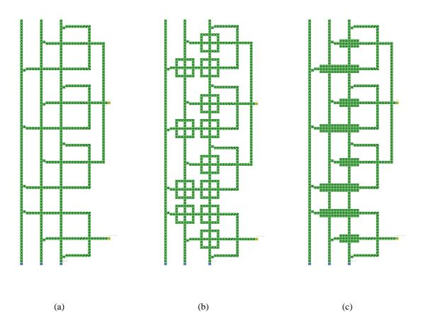
Fig. 18. Full adder (a) Xb crossings (b) TMRXb crossings (c) ThickXb crossings.
