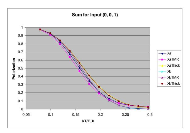
Fig. 20. Full Adder: Thermal performances on the Sum output
