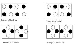
Fig. 11. Configuration energies for normal (top row) and rotated (bottom row) cells. (the lowest energy configurations on the left, the highest energy configurations on the right)
