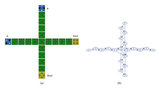
Fig. 5. Normal crossing with rotated central cell (Xa) (a) Layout (b) BN with 2-cell radius of influence.
