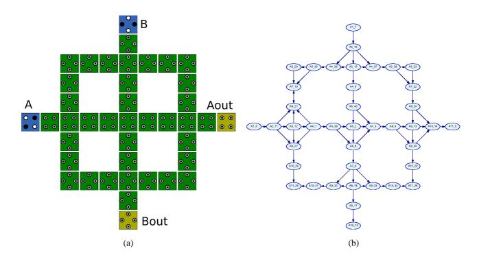
Fig. 7. 3x1 TMR crossing with non rotated central cell (TMRXb voting on the B line) (a) Layout (b) BN with 2-cell radius of influence.
