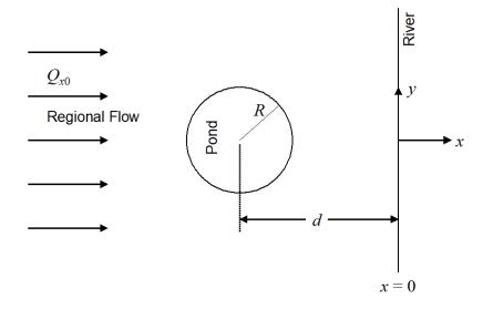
(1) Write the expression for the discharge potential,  $\Phi(x, y)$ , of the groundwater. The hydraulic head at the river is h = 10 m. (The river is a constant-head boundary.)
