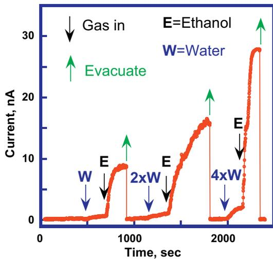
**Fig. 5.** Sensor current response of a single nanobelt SnO<sub>2</sub> device to 20 ppm ethanol when the chamber is pre-filled with 25 ppm, 50 ppm, and 100 ppm of water, respectively.
