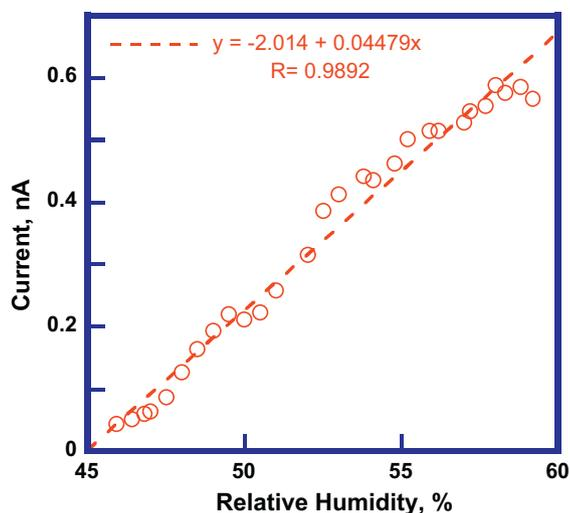
Fig. 3. SnO<sub>2</sub> nanobelt current linear dependence on air humidity.
