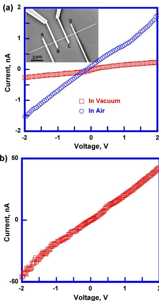
**Fig. 2.** (a) Current–voltage characteristics of an individual  $\text{SnO}_2$  nanobelt in air and in vacuum. The inset is an SEM image of the  $\text{SnO}_2$  nanobelt sensing device; (b) improved conductivity after  $200^\circ\text{C}$  thermal treatment measured in vacuum.
