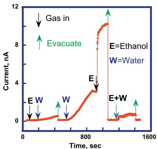
Fig. 4. Water and ethanol current response of SnO<sub>2</sub> single nanobelt device. E, W and E and W correspond to 20 ppm ethanol, 25 ppm water and a mixture of 20 ppm ethanol and 25 ppm water, respectively.
