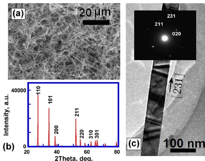
**Fig. 1.** (a) SEM image of  $\text{SnO}_2$  nanobelts; (b) XRD pattern of as-grown  $\text{SnO}_2$  nanobelts; (c) TEM image and electron diffraction pattern (inset) of an individual nanobelt showing  $[231]$  growth direction. The top nanobelt surface is  $(\bar{1}02)$  or  $(10\bar{2})$ .
