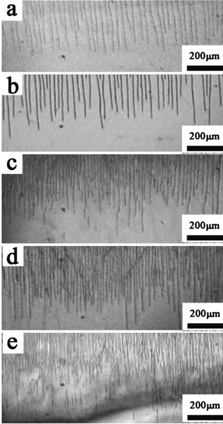
FIG. 3. Optical images of the cracks spacing of the films formed of different radii spheres: (a)  $R=85$  nm, Cracks spacing  $W \approx 15.6 \pm 0.77$   $\mu\text{m}$ ; (b)  $R=110$  nm,  $W \approx 12.5 \pm 0.55$   $\mu\text{m}$ ; (c)  $R=150$  nm,  $W \approx 8.86 \pm 0.42$   $\mu\text{m}$ ; (d)  $R=180$  nm,  $W \approx 8.17 \pm 0.44$   $\mu\text{m}$ ; (e)  $R=215$  nm,  $W \approx 7.53 \pm 0.50$   $\mu\text{m}$ .
