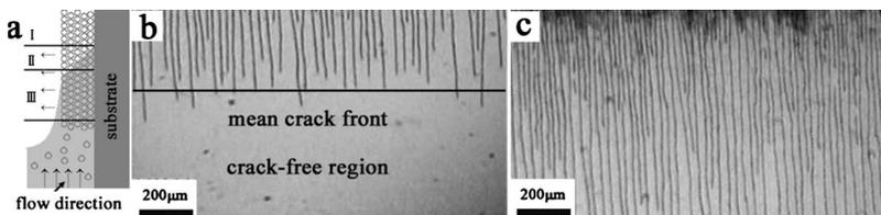
FIG. 2. (a) Schematic drawing of the film growth: I dried region; II partially dried region; III saturated region; (b) optical image of the colloidal crystal formation ( $R=110$  nm); (c) optical image taken 2 h after b.
