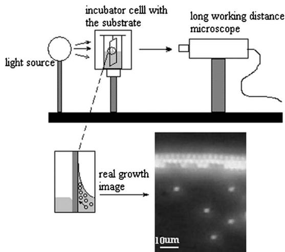
FIG. 1. A schematic of the experimental setup. A magnified schematic of the observed region is shown at the vicinity of the meniscus, as well as the image observed at the initial growing stage. Large colloid spheres with the diameter of 3 micrometers were used in the observation of the initial assembly process.
