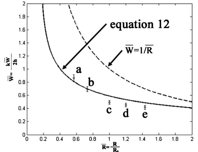
FIG. 6. Theoretical relationship between  $\bar{W}$  and  $\bar{R}$ . Points a–e are the experimental values for 85, 110, 150, 180, or 215 nm particles radii, respectively. (a)  $\bar{R}=0.57$ ,  $\bar{W}=0.87 \pm 0.05$ ; (b)  $\bar{R}=0.73$ ,  $\bar{W}=0.69 \pm 0.04$ ; (c)  $\bar{R}=1.00$ ,  $\bar{W}=0.49 \pm 0.03$ ; (d)  $\bar{R}=1.20$ ,  $\bar{W}=0.45 \pm 0.03$ ; (e)  $\bar{R}=1.43$ ,  $\bar{W}=0.42 \pm 0.03$ .  $1/\bar{R}$  trend line is added for comparison.
