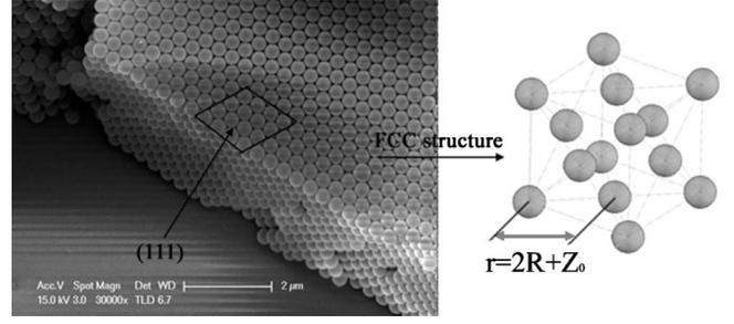
FIG. 5. FCC structure of the film.
