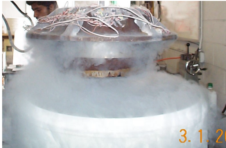
Figure 7.18 Cooled hub pulled out of the dewar.
