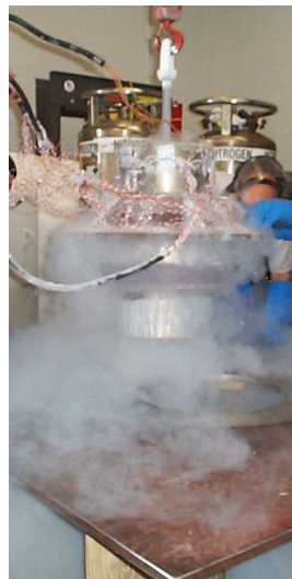
Figure 7.13 Insertion of cooled trunnion-hub into the girder.
