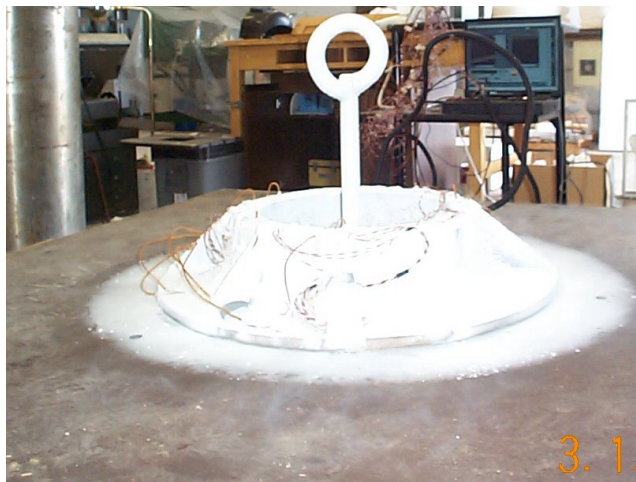
Figure 7.21 Hub-girder sub-assembly (Step 2 completed).
