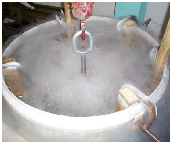
Figure 7.23 Trunnion cooled in the liquid nitrogen dewar.
