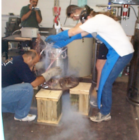
Figure 7.8 Insertion of cold trunnion into the hub (Step 2 of AP1).
