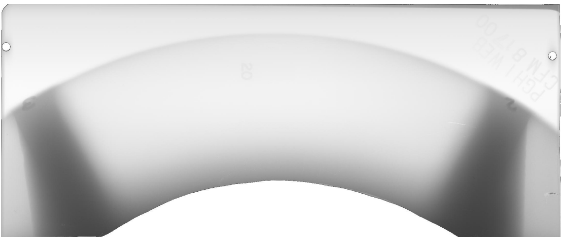
Figure D.2c X-ray of the hub from the web view (2-3).
