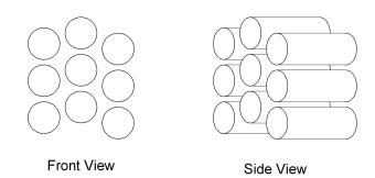
This is a pretty good (not perfect) model of the pores in a porous medium. Suppose each tube has a radius R and a length L. There is a pressure gradient  $\Delta P$  across the bundle of tubes. Water flows through the tubes in response to this pressure gradient. You may assume that the flow is laminar, and you may treat the water as incompressible. We can use this model to investigate the permeability of porous media.
