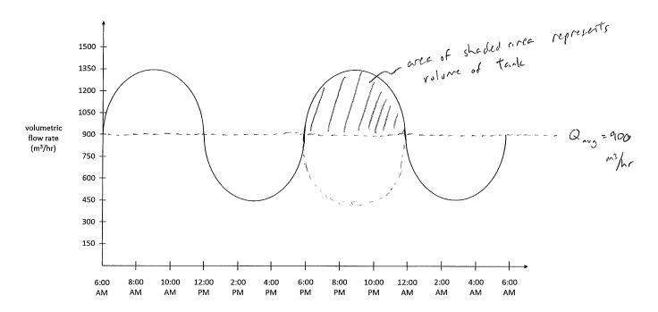
You want to design a flow equalization basin to smooth out the flow rate, so that the rest of the plant can operate at (or close to) steady state.
