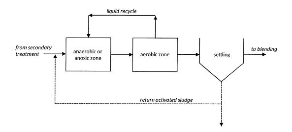
a. (10 pts) Because you took ENV 4417, you realize that this system will probably not work for nitrogen removal at the treatment plant being proposed for Sprawlville. Explain why not. Hint: look at where the nitrogen removal process is located in the Sprawlville plant; what will *not* be present at that point in the treatment train?
