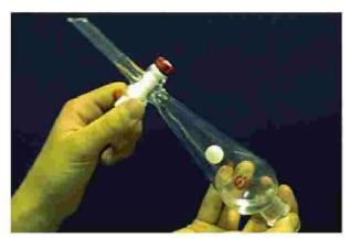
point the stem up and away from you when you open the stopcock to release pressure
