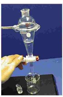
3. After the layers have separated completely, be sure the stopper is out; then open the stopcock and allow the lower layer to drain into the flask.
