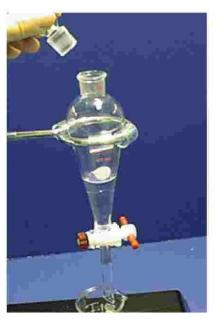
2. While waiting, place a beaker under the funnel. If the solvent is not too volatile, you can remove the stopper.
