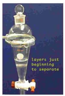
1. Let the funnel rest undisturbed until the layers are clearly separated.
