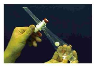
Vent frequently to prevent pressure buildup, which could cause the stopcock (and perhaps hazardous chemicals) to blow out. Take special care when washing acidic solutions with bicarbonate or carbonate since this produces a large volume of CO<sub>2</sub> gas.
