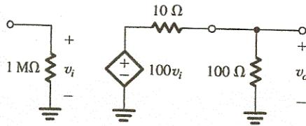
$$\begin{aligned} A_v &= \frac{v_o}{v_i} \\ &= 100 \times \frac{100}{100 + 10} \\ &= 90.9 \text{ V/V} \end{aligned}$$
