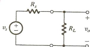
$$\frac{v_o}{v_s} = \frac{R_L}{R_L + R_s}$$
