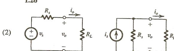
$R_L$  represents the input resistance of the processor
