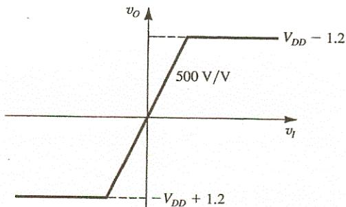
For  $V_{DD} = 10 \text{ V}$ , the largest undistorted sine-wave output is of 8.8-V peak amplitude or  $6.2 \text{ V}_{\text{rms}}$ . Input needed is  $12.4 \text{ mV}_{\text{rms}}$ .
