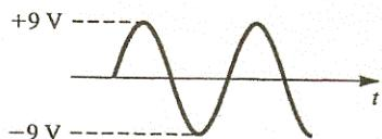
(b) For an output that is clipping 90% of the time,  $\theta = 0.1 \times 90^\circ = 9^\circ$  and  $V_p \sin 9^\circ = 9 \text{ V} \Rightarrow V_p = 57.5 \text{ V}$  which of course does not occur as the output saturates at  $\pm 9 \text{ V}$ . To produce this result, the input peak must be  $57.5/1000 = 57.5 \text{ mV}$ .
