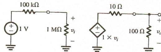
$$\begin{aligned} v_o &= 1 \text{ V} \times \frac{1 \text{ M}\Omega}{1 \text{ M}\Omega + 100 \text{ k}\Omega} \times 1 \times \frac{100 \Omega}{100 \Omega + 10 \Omega} \\ &= \frac{1}{1.1} \times \frac{100}{110} = 0.83 \text{ V} \end{aligned}$$
