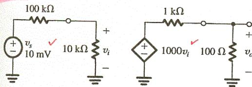
$$\begin{aligned} \frac{v_o}{v_s} &= \frac{10 \text{ k}\Omega}{10 \text{ k}\Omega + 100 \text{ k}\Omega} \times 1000 \times \frac{100 \Omega}{100 \Omega + 1 \text{ k}\Omega} \\ &= \frac{10}{110} \times 1000 \times \frac{100}{1100} = 8.26 \text{ V/V} \end{aligned}$$
