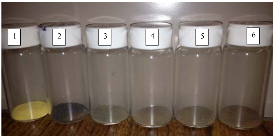
Figure 1: Shows the synthesized catalysts. (1) Ceria Zirconia support, (2) Support with nickel and magnesium loadings, (3-6) Support with 1:1 nickel:magnesium and various platinum loadings.
