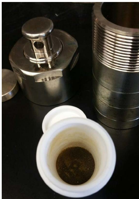
Figure 3: Catalyst poisoned in autoclave
