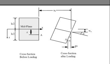
Relationship between displacements through the thickness of a plate to midplane displacements and curvatures.
