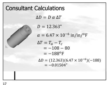
Is the  $\Delta D = D\alpha \Delta T$  formula correct?  $\alpha$  ( $\mu$ in/in/ $^{\circ}$ F)  $T({}^{\circ}\mathsf{F})$ -340 2.45 -300 3.07 -220 4.08  $\alpha$  ( $\mu$ in/in/F) -160 4.72 5.43 -80 6.00 0 6.24 40 Temperature (F) 80 6.47 18
