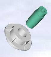
After Cooling, the Trunnion Got Stuck in Hub
