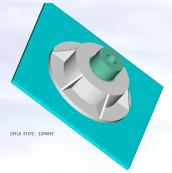
**Step1.** Trunnion immersed in dry-ice/alcohol
