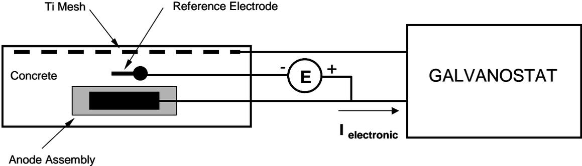
Fig. 2: Anode Test Arrangement (Idealized-Actual Placement May Vary)
