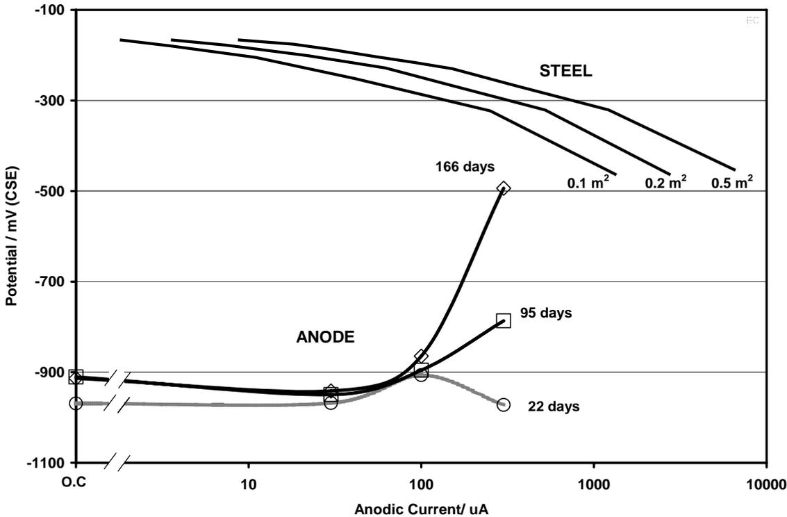
Fig. 3: Illustration of preliminary findings for one of the anode types investigated, with superimposed abstracted cathodic polarization behavior of passive rebar (Sagüés et al 2003), adjusted for total steel area as indicated. Times indicated are since first energizing the system.
