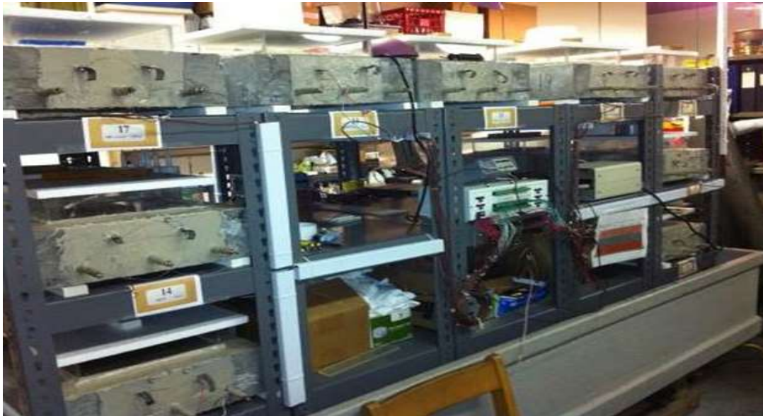
Figure 2: Testing arrangement for cracked concrete specimens.
