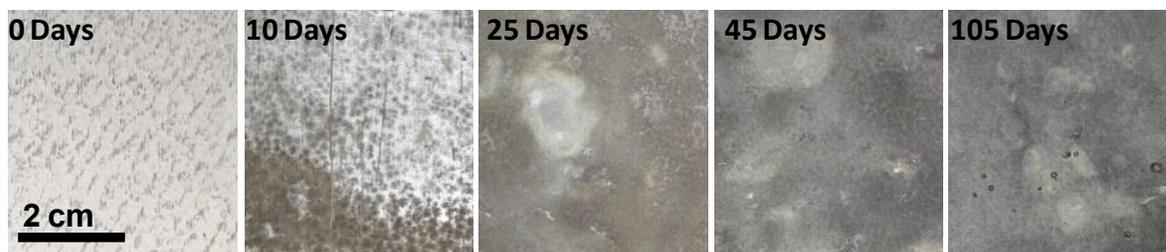
Figure 3: Surface discoloration over time; pits with rust were observed around 150 days of exposure.
