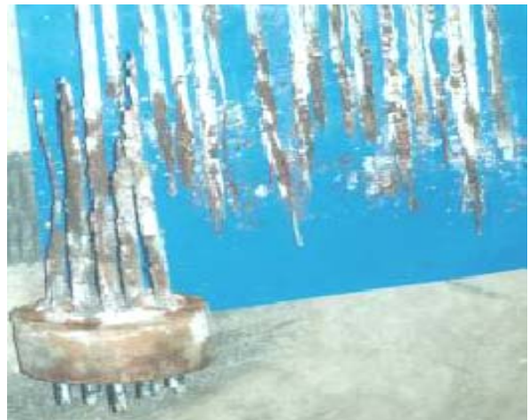
FIGURE 2 Severe Failure of Post-Tensioning Tendons near Cap Region (Corven, 2001) a) Failed tendon at Niles Channel Bridge b) Failed tendon at Column 133 NB of Sunshine Skyway Bridge
