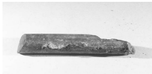
FIGURE 3- Extracted spiral wire, severe corrosion. Spiral wire from P149-2, 0.64 cm diameter, showing appreciable localized loss of cross section at the right end of the segment cut out by coring.
