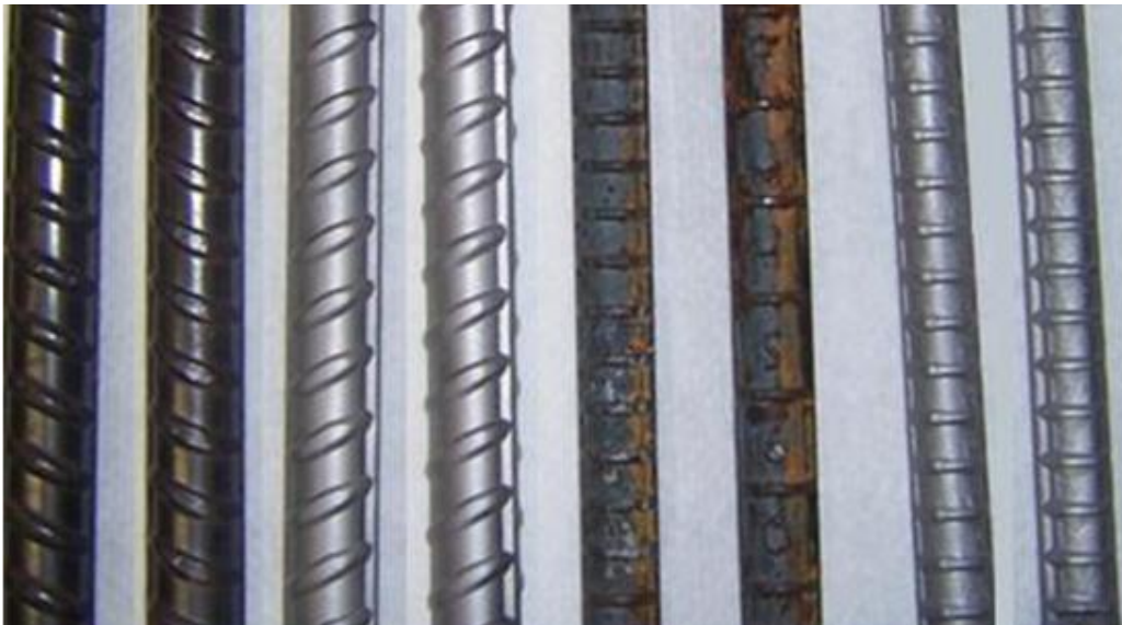
Figure 2: Appearance of duplicate specimens [from left to right: As-received 9%Cr, Surface blasted 9%Cr, As-received CS, Surface blasted CS].
