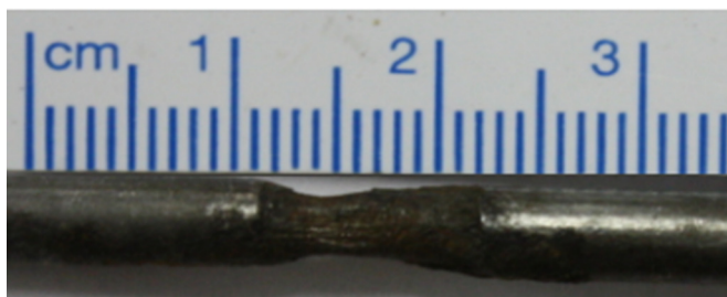
Figure 7: Corrosion influence zone at a wire-0.1 inch (2.5 mm) crack intersection of R12 after 246-day exposure to continuous and cyclic 500 ppm chloride environment
