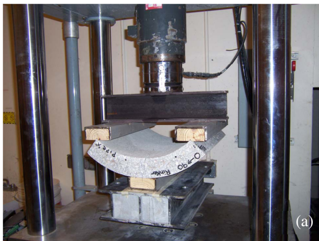
Figure 3: (a) Cracking rig used to generate cracks in RC culvert pipe specimens, (b) Top view for 0.01 in (~2.5 mm) Z-type specimen showing Crack width measurement along a crack using a crack comparator.
