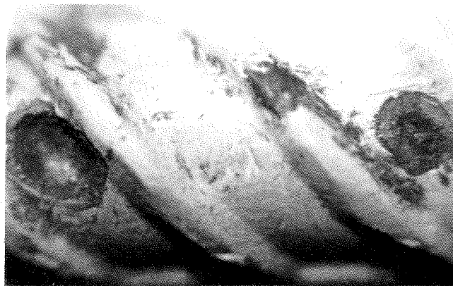
FIGURE 8 - Appearance of the surface after removing disbonded coating from a specimen exposed to Solution Type III (calcium hydroxide plus sodium chloride) for one month at -400 mV vs SCE.
