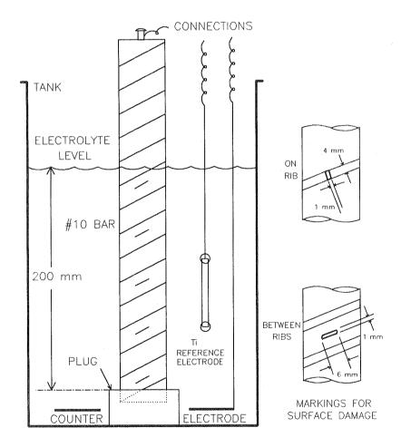
FIGURE 4 - Specimen and electrode setup for the potentiostatic exposures.
