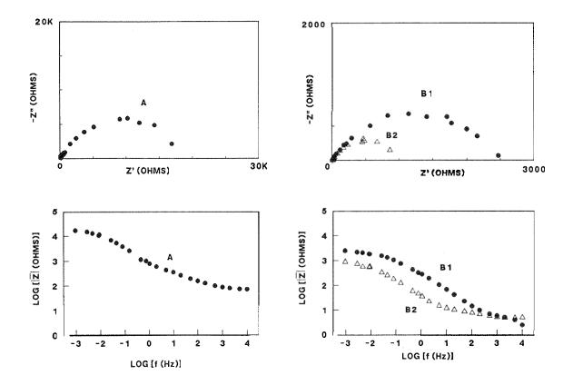
FIGURE 7 - EIS behavior of specimens in the sodium chloride solution (Type II). A) Material in the as-received condition, one month of exposure.
