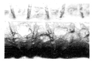
FIGURE 2 - Appearance of a #5 reinforcing bar (horizontal hoop portion of a bridge substructure column) after sandblasting.
