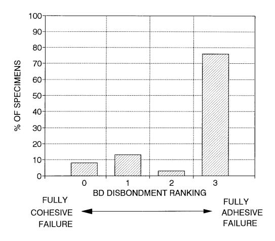
Figure 1. Knife disbondment test results for dry specimens (Mode BD disbondment rating)
