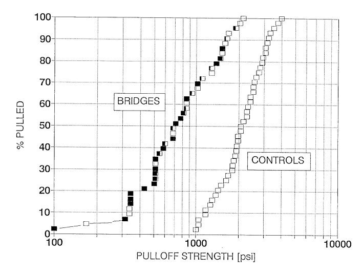
Figure 2. Distribution of the pulloff strength of ECR specimens extracted from the field bridge sites and of unexposed controls (Ref.[2]). Completely filled symbols indicate total epoxy-base metal separation under the test dolly. Partial filling is proportional to fraction separated. (1,000 psi = 6.895 MPa).
