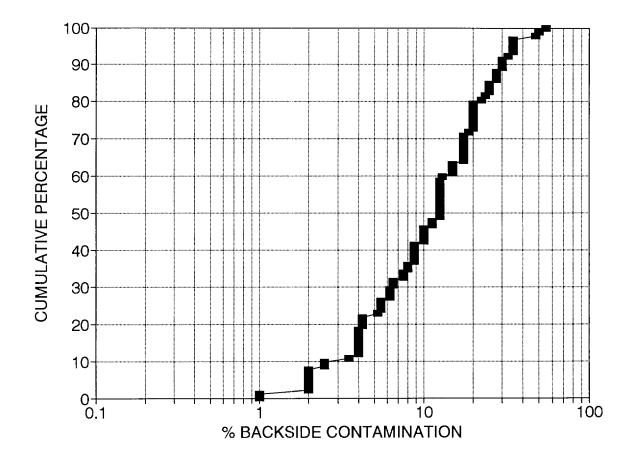
Figure 3. Distribution of the % backside contamination in field-extracted samples with BD rating  $\ge 1$ .
