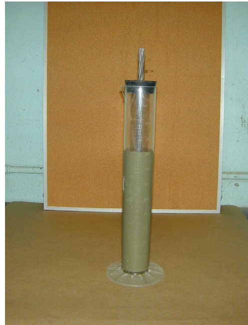
Figure 7 – Photograph of the test apparatus for measuring grout bleed-water and grout volume change.
