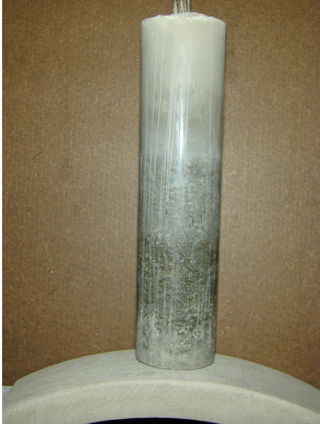
Figure 8 – Photograph depicting increasing chalkiness toward the top of the aluminum admixed grout (vibrated).
