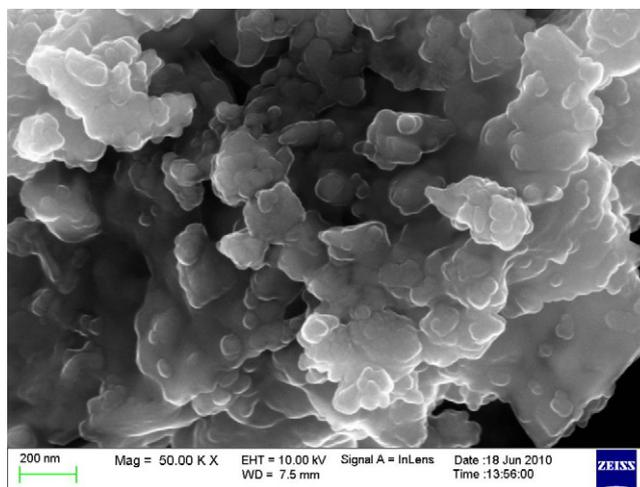
Fig. 5. FE-SEM micrograph of  $\text{Fe}_3\text{O}_4$  nanoparticles heated at  $700^\circ\text{C}$  for 2 h.
