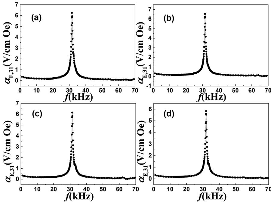
FIG. 2. The frequency dependence of  $\alpha_{E,31}$  in parallel mode when  $H_{DC} = 700$  Oe (a) 1 PZT; (b) 2 PZT plates; (c) 3 PZT plates; and (d) 4 PZT plates.
