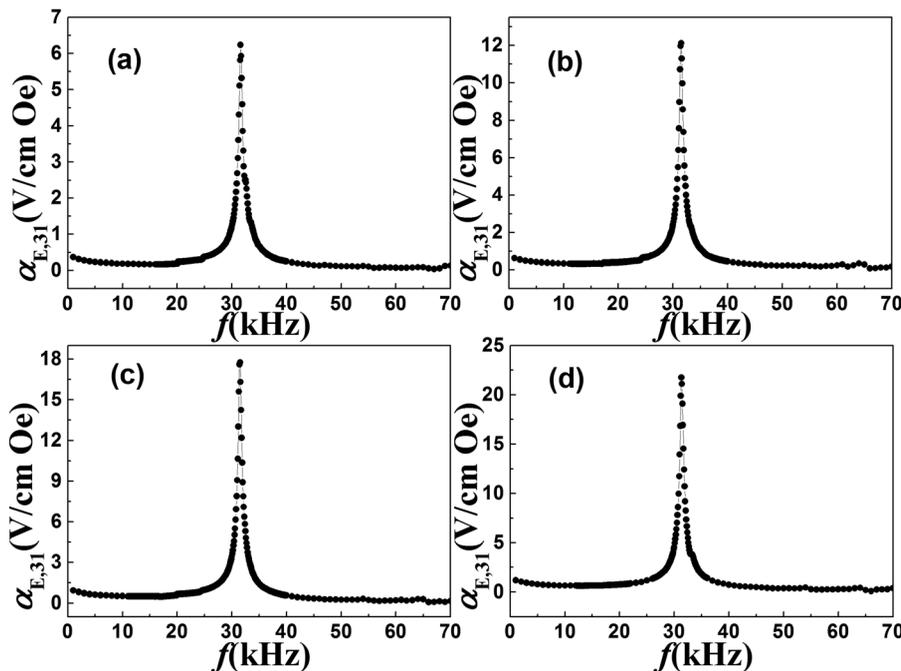
FIG. 3. The frequency dependence of  $\alpha_{E,31}$  in serial mode when  $H_{DC} = 700$  Oe (a) 1 PZT; (b) 2 PZT plates; (c) 3 PZT plates; and (d) 4 PZT plates.
