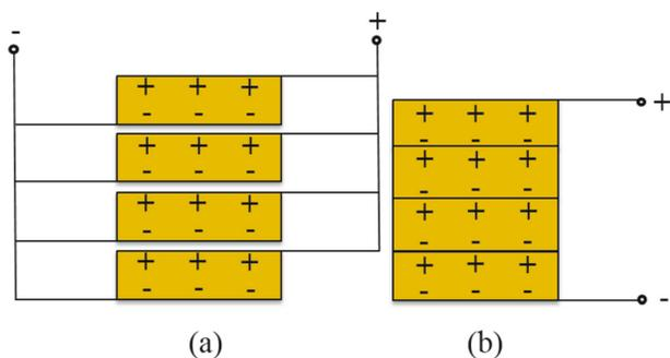
FIG. 4. The sketch map of (a) parallel mode and (b) serial mode.
