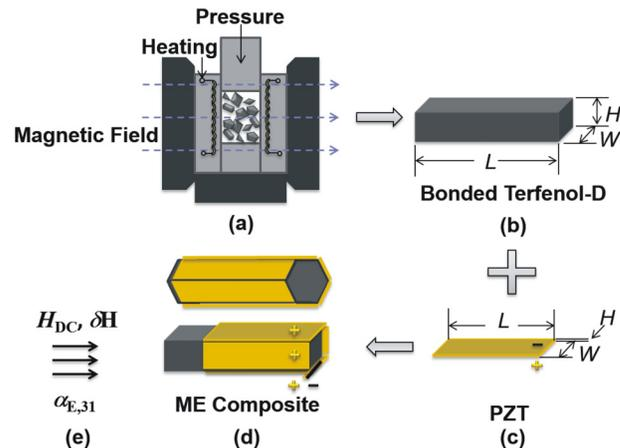
FIG. 1. The illustration of preparation process and ME measurement of the bonded Terfenol-D/ $\text{Pb}(\text{Zr},\text{Ti})\text{O}_3$  ME composites.
