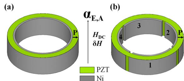
FIG. 1. Schematic illustration of (a) PZT/Ni cylinder; (b) PZT/Ni cylinder with arrayed Ni arc layers.
