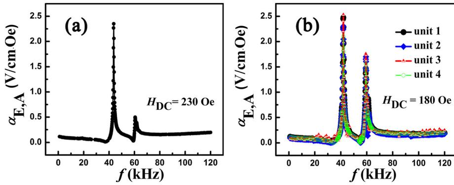
FIG. 2. The ME voltage coefficient,  $\alpha_{E,A}$ , dependence on the applied magnetic field frequency: (a) PZT/Ni cylindrical layered composite with  $H_{DC} = 230$  Oe; (b) each of the four units of the PZT/Ni cylinder with quarter arrayed Ni arc layers with  $H_{DC} = 180$  Oe.
