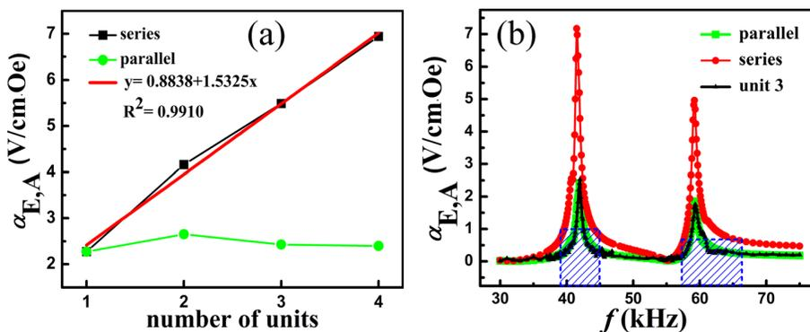
FIG. 3. (a) The maximum ME voltage coefficient,  $\alpha_{E,A}$ , as a function of the number of units connected either in series or in parallel; (b) the frequency dependence of  $\alpha_{E,A}$  with  $H_{DC} = 180$  Oe for the unit 3 alone and all the four units connected either in series or in parallel.
