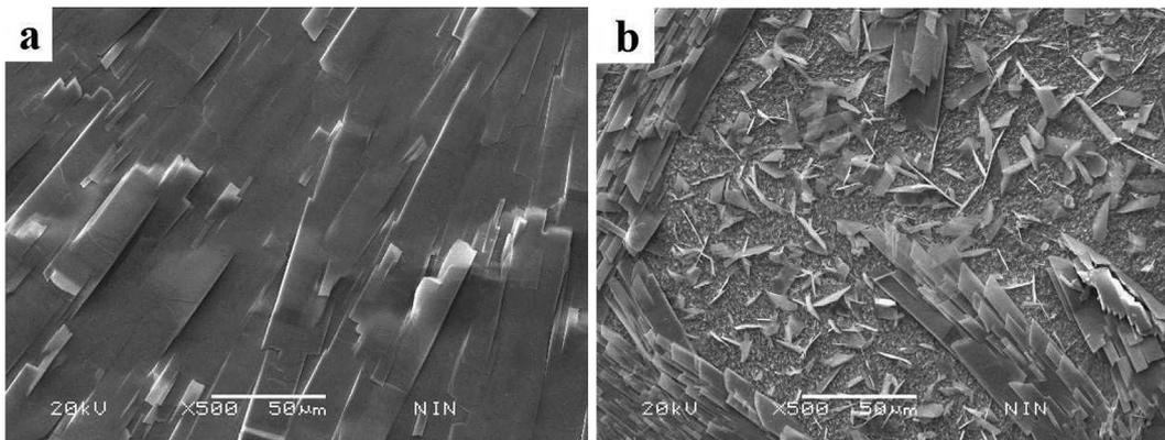
Fig. 5. SEM images of the La-TZM samples surface oxidized at: (a) 1000 °C, 10 min and (b) 1000 °C, 15 min [9].
