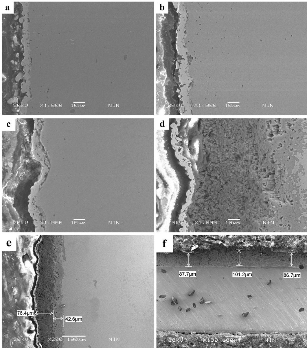
Fig. 7. Cross-sectional SEM images of Pt-coated La-TZM alloy plates heated at different temperature and different times: (a) 400 °C, 4 h; (b) 600 °C, 4 h; (c) 800 °C, 15 min; (d) and (e) 800 °C, 4 h and (f) La-TZM alloy plate heated at 800 °C for 10 min [9].
