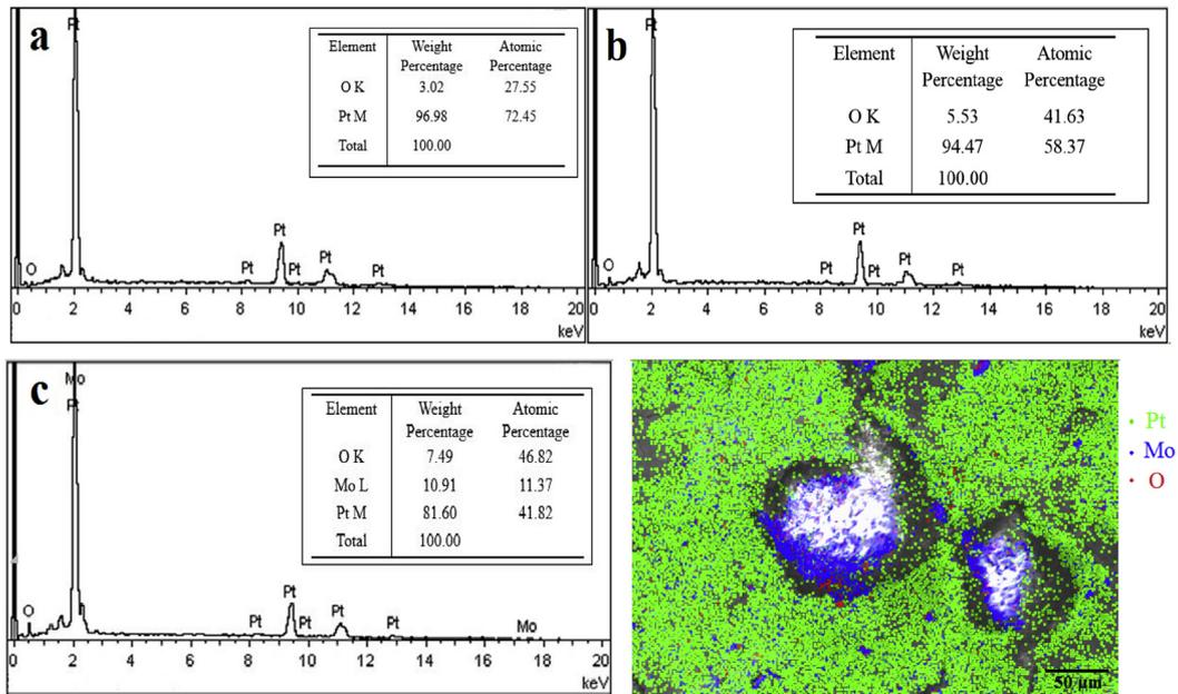
Fig. 4. Surface EDS profiles of the samples oxidized in 4 h at different temperature: (a) 400 °C; (b) 600 °C; (c) 800 °C.
