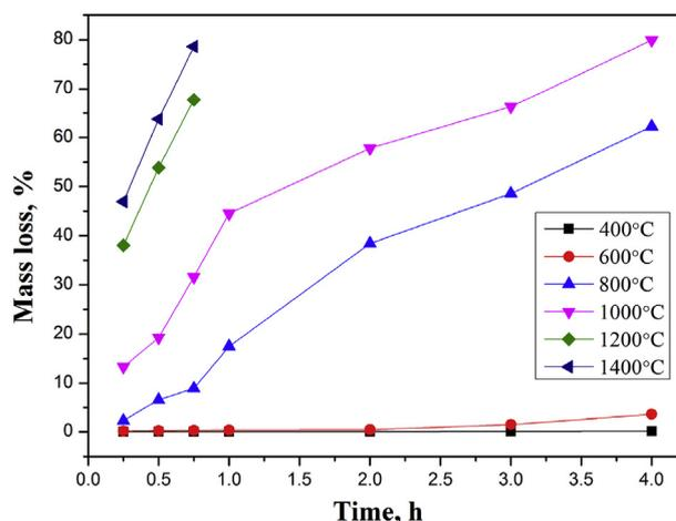
**Fig. 1.** Oxidation mass loss of the samples tested at different temperature.
