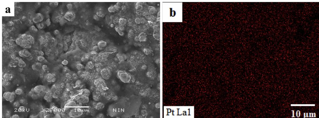
Fig. 2. (a) SEM and (b) EDS elements analysis images of the original sample Pt-coated surface.
