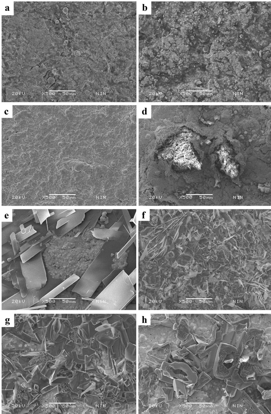
**Fig. 3.** SEM images of the Pt-coated La-TZM samples surface oxidized at different temperature and time: (a) 400 °C, 4 h; (b) 600 °C, 4 h; (c) 800 °C, 15 min; (d) 800 °C, 4 h; (e) 1000 °C, 15 min; (f) 1000 °C, 4 h; (g) 1200 °C, 15 min; and (h) 1400 °C, 15 min.
