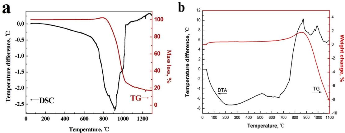
Fig. 8. TG-DTA/DSC curves of TZM alloy plates: (a) Pt-coated La-TZM alloy; (b) La-TZM alloy.
