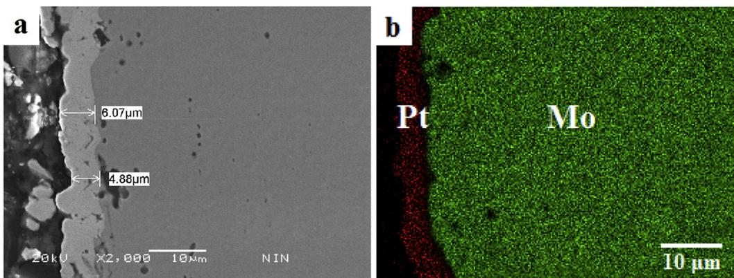
Fig. 6. Cross-sectional SEM and EDS images of the Pt-coated La-TZM alloy plate.
