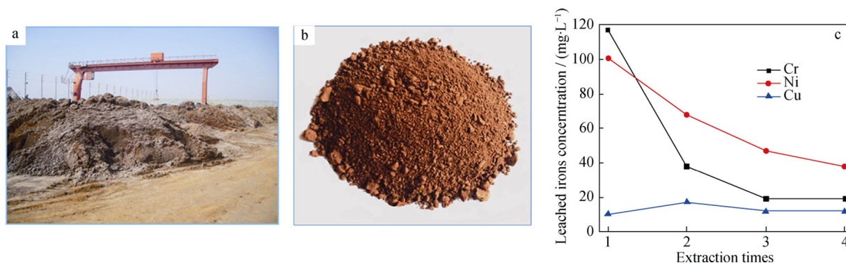
Fig. 1 Open-air depot of PS a , dried PS b , and leaching concentration of heavy metals of the PS, depending on number of leaching times c
