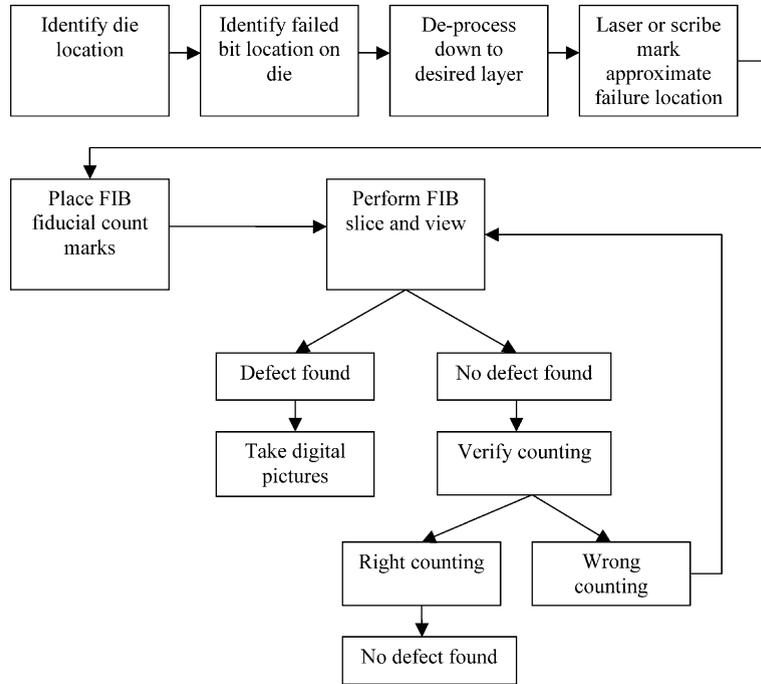
Fig. 7. Block diagram of the FIB failure analysis.
