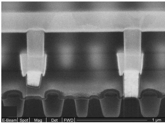
Fig. 8. SEM images of via contacts from transistors to second level metallization. The etch used to create the via on the left was incomplete, resulting in an electrical open.
