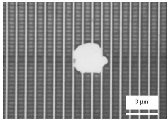
Fig. 2. An optical image of a cluster defect (particle) magnified by the upper layers.
