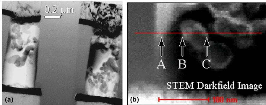
Fig. 13. (a) A TEM bright-field image of a pair of vias from a multiple bit failure site where the bits were electrically open. There is no metal via-fill, and clusters of particles are present in the vias. (b) STEM dark-field image of some particles in the bottom left corner of the right via, where EDS–PEELS spectrum profiling was performed. Three positions of the electron probe are labeled along the profile.
