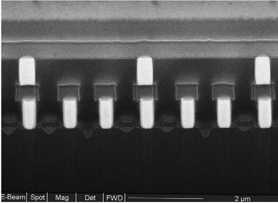
Fig. 5. SEM view of three transistor pairs.
