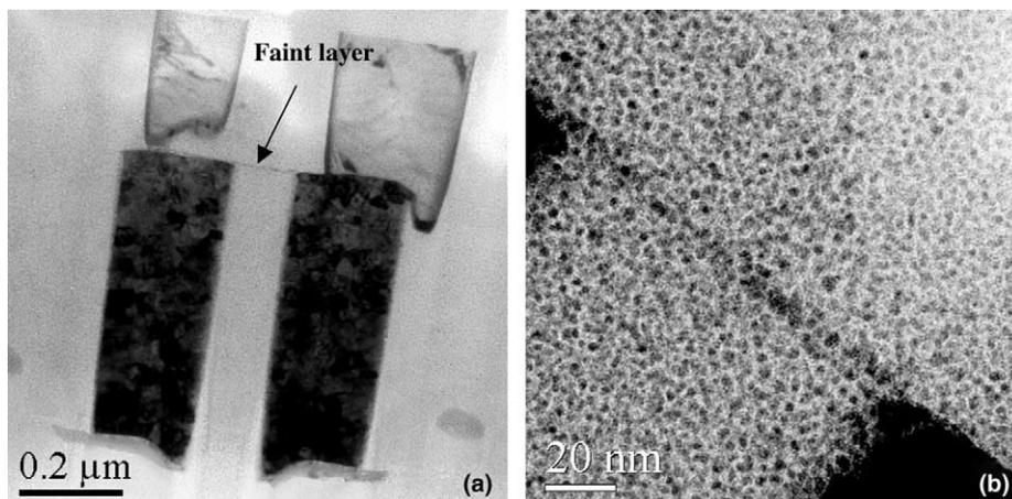
Fig. 11. (a) TEM image of a pair of tungsten plugs in a shorted bit. A faint dark layer between the tungsten plugs is noticeable. (b) A higher magnification view of the faint layer in (a). The dark layer is residual titanium that was left behind by the CMP (chemical-mechanical planarization).
