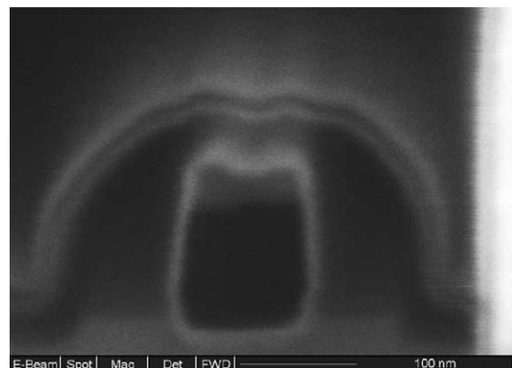
Fig. 4. High-resolution FIB SEM image showing polysilicon spacer.
