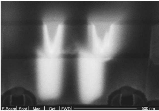
Fig. 6. SEM image showing a defect shadow before milling through it. Here, the FIB cut surface is tilted  $38^\circ$  to the SEM beam, which allows seeing a thin in-plane defect projection.
