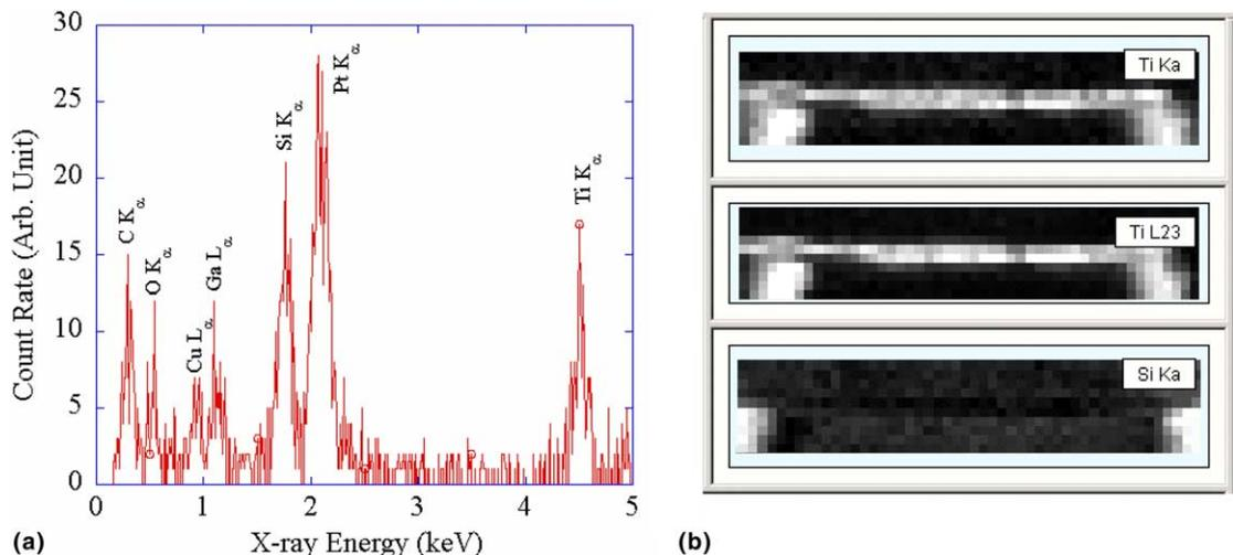
Fig. 12. (a) An EDS spectrum acquired from the faint layer between the two W-plugs. (b) Elemental maps of Ti based on integrated intensities of the Ti K $\alpha$  X-ray and the Ti L<sub>2,3</sub> edge, and the Si K $\alpha$  X-ray.
