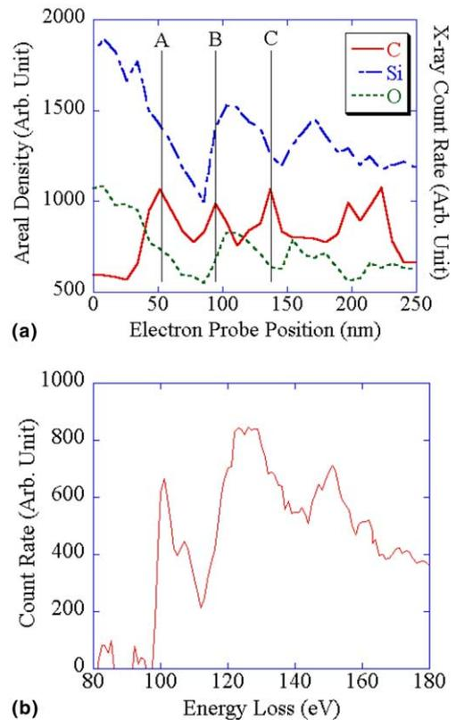
Fig. 14. (a) Profiles of the areal densities of C (acquired from PEELS), Si and O (obtained from integrated intensities of their  $K\alpha$  X-rays). (b) The  $L_{2,3}$  edge of Si observed from the particle between positions B and C of the electron probe.
