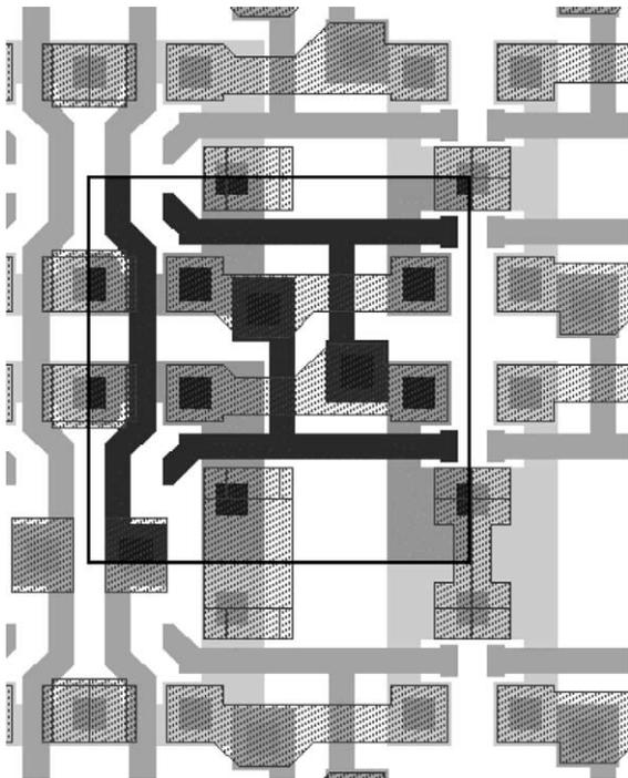
Fig. 1. Schematic of a bit cell containing six transistors.
