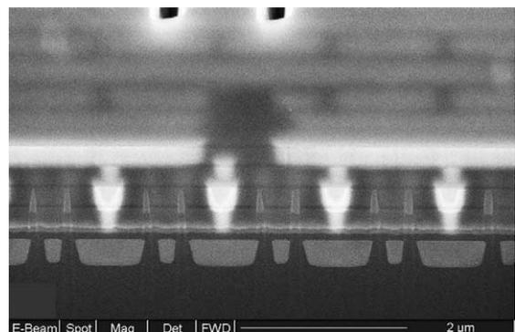
Fig. 9. SEM image of two open bits due to a pattern defect.
