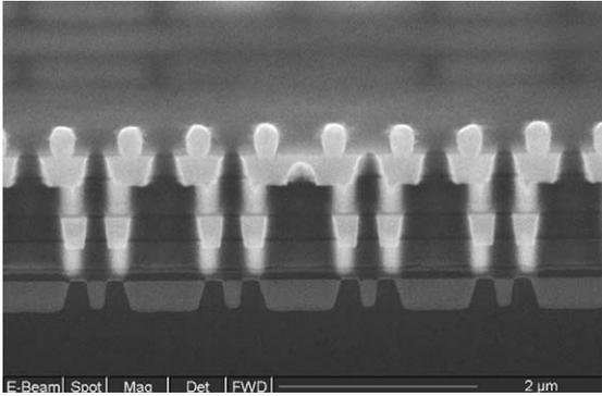
Fig. 10. SEM image of shorted bits. Here, second metal lines in the middle are bridged together.
