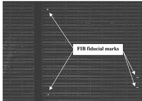
Fig. 3. Top-down FIB image of a memory array showing fiducial counting marks.
