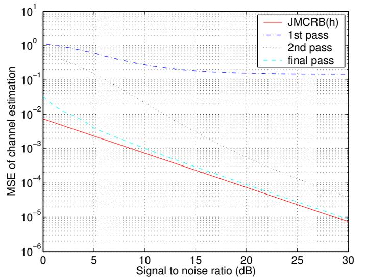
Figure 4: Mean square error performance of channel estimation algorithm for a normalized frequency offset of 1. Joint modified Cramér-Rao bound is also shown.
