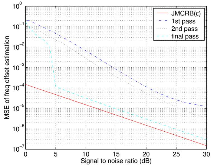
Figure 3: Mean square error performance of frequency offset estimation algorithm for a normalized frequency offset of 1. Joint modified Cramér-Rao bound is also shown.
