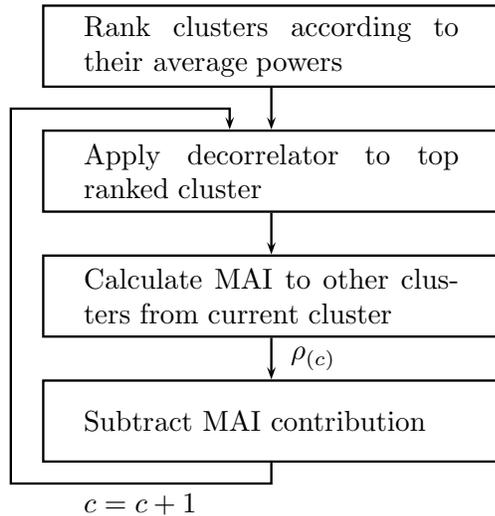
Fig. 1. Block diagram of the proposed compensation algorithm.
