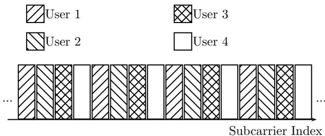
Fig. 1. Illustration of subcarrier allocation in clustered OFDMA.
