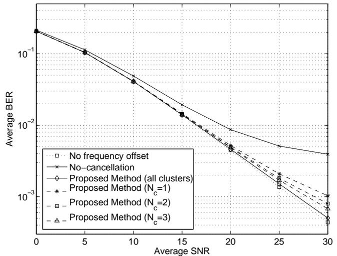
Fig. 3. Uncoded bit error rate (BER) as a function of average SNR. The normalized frequency offset has a uniform distribution in the range (-0.1, 0.1).
