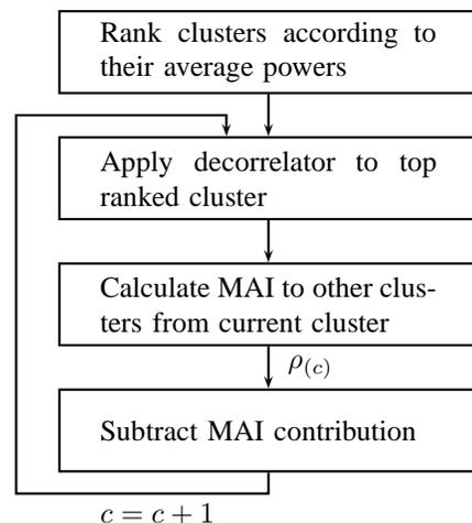
Fig. 2. Flow chart of the proposed compensation algorithm.
