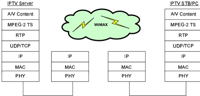
Fig. 2. Protocol Stack for IPTV Transmission.
