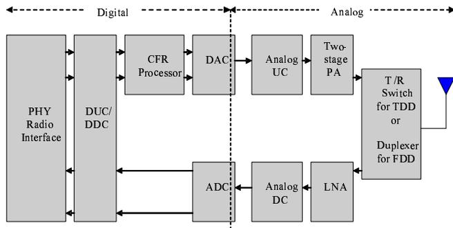
Fig. 5. Block diagram of WiMAX BS Radio Transceiver.
